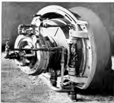
Ray rotary fuel oil burner of the turbine drive type recently installed on a San Francisco ocean-going tug
